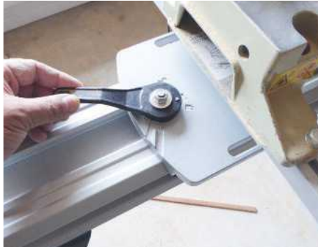
▲ These levers have the job of locking the saw brackets to the stand
